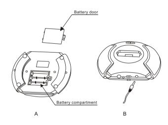
① A. Install 3pcs AA batteries(not included) into battery compartment or use DC 9V adapter
